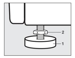
Use the combination wrench provided to turn the counternut 2 counterclockwise. Then turn the counter nut 2 together with the foot 1 to unscrew. ■ Use a level to check that the washer is standing square.
